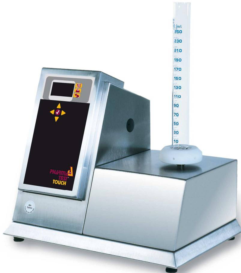
**PT-TD200 Touch** is a single station testing instrument to test the Apparent Volume and Apparent Density of powders and granules in compliance with USP <616 App. 1 + 2> and also with the EP <2.9.34> and DIN 53194 in one instrument. The electronics automatically detects in which position the cylinder dish has been introduced and adjust the tapping speed and height according to the requirements of EP/USP 616, Method II or USP 616, Method 1
